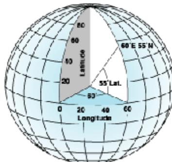
In the spherical system, horizontal lines, or east–west lines, are lines of equal latitude, or parallels. Vertical lines, or north–south lines, are lines of equal longitude, or meridians. These lines encompass the globe and form a gridded network called a graticule.
