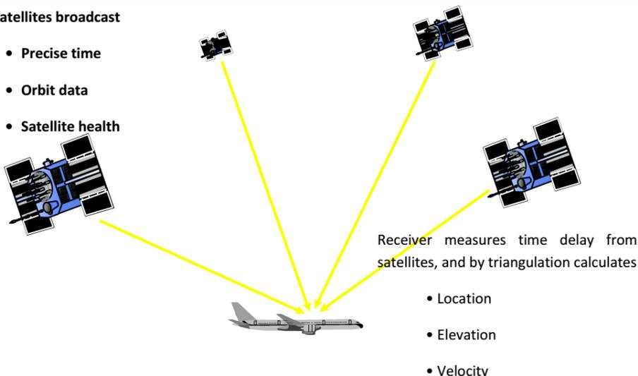
GPS is a system. It's made up of three parts: satellites, ground stations, and receivers. Satellites act like the stars in constellations—we know where they are supposed to be at any given time. The ground stations use radar to make sure they are actually where we think they are. A receiver, like you might find in your phone or in your parents car, is constantly listening for a signal from these satellites. The receiver figures out how far away they are from some of them.
